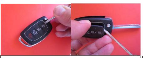
**Do Not open remote.** Gently remove an old rubber pad from your remote using flat screw driver.
