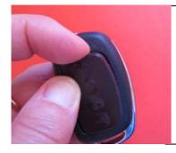
Place a new silicone pad over top part of your remote. Use rolling motion when positioning pad in grooves and press firmly till pad "engages" with hard shell all around edges. DO NOT USE any lubricants or detergents for cleaning grooves as it will affect firm seating of a pad. **No re-programming is required.**
