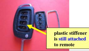
If after removing old pad your remote looks like in the picture <u>above</u> than <u>you</u> need to remove, <u>plastic stiffener still</u> <u>attached</u> to your remote. Use small flat screwdriver to lift it up and detach it from remote. It will not be used as new Silicone buttons does not need extra support.
